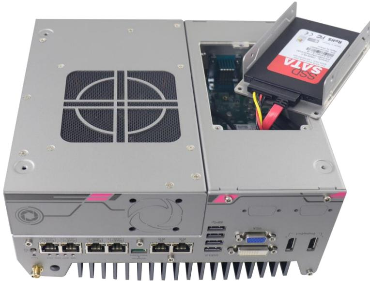
5. Gently wiggle the bracket back into the enclosure and secure it with three (3) M3 flat-head screws.
