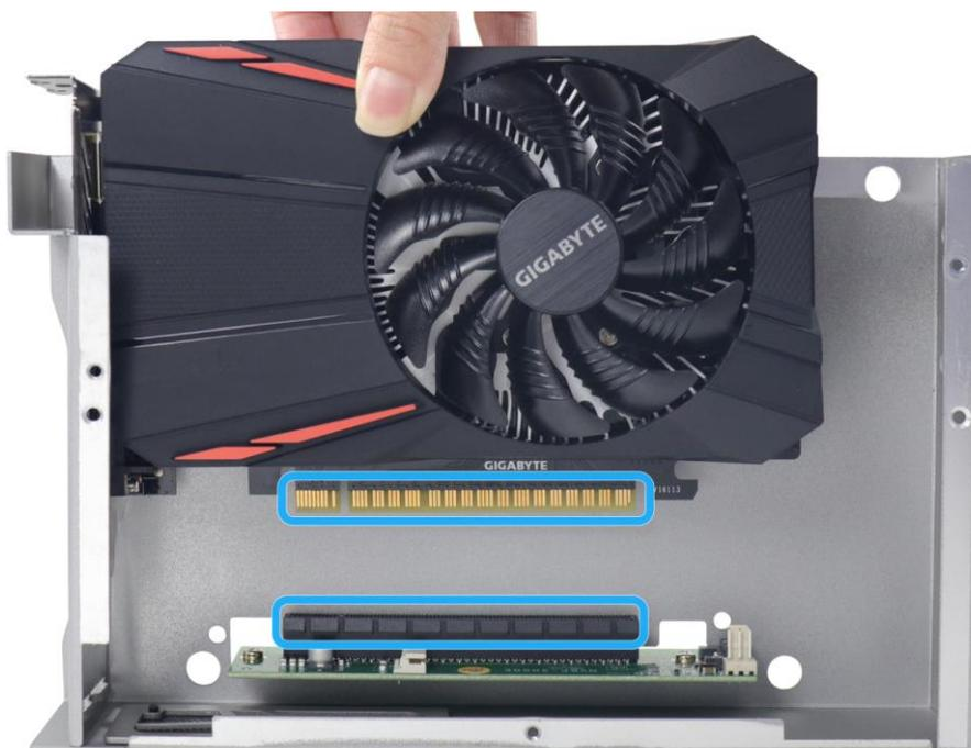
3. Make sure the bottom of the graphics card slot cover is properly inserted into the hinge on the enclosure.
