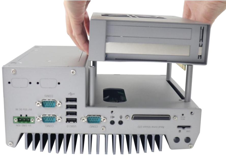
5. Secure the Cassette module by securing the four (4) screws.
