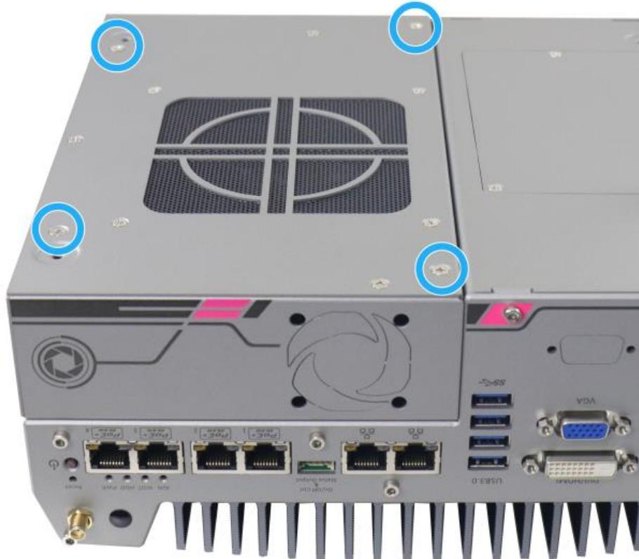
3. Gently lift and separate the Cassette enclosure from the system enclosure.
