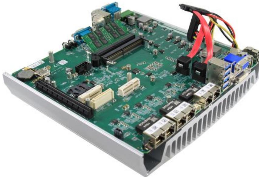
4. Push down on the edge of the module and the clips on the side should clip the module into place.
