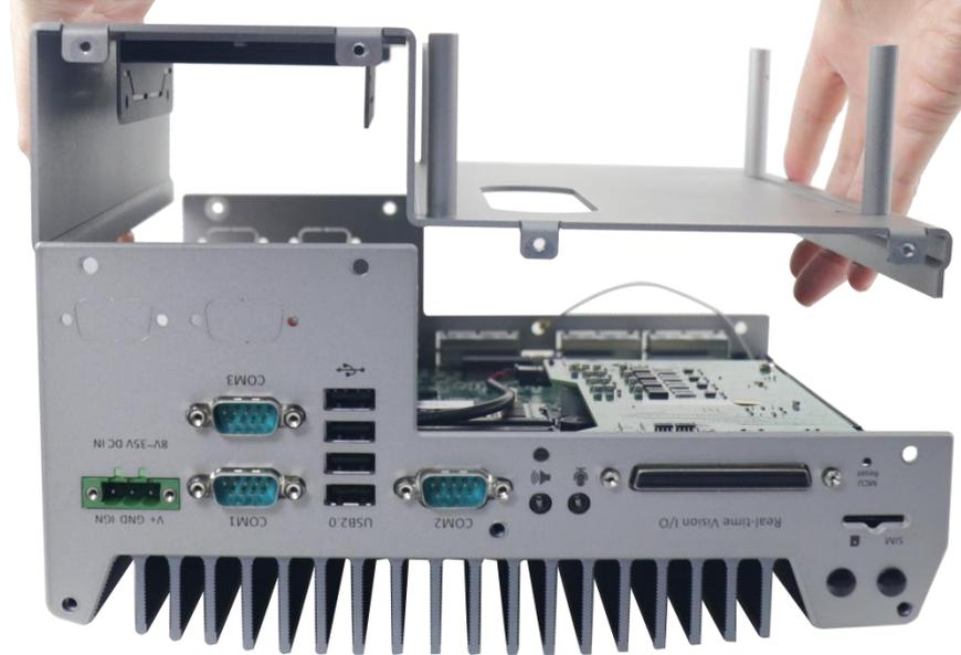
2. Secure the seven (7) screws on the front panel.
