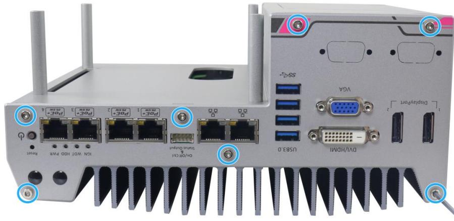
3. Secure the seven (7) screws on the rear panel.
