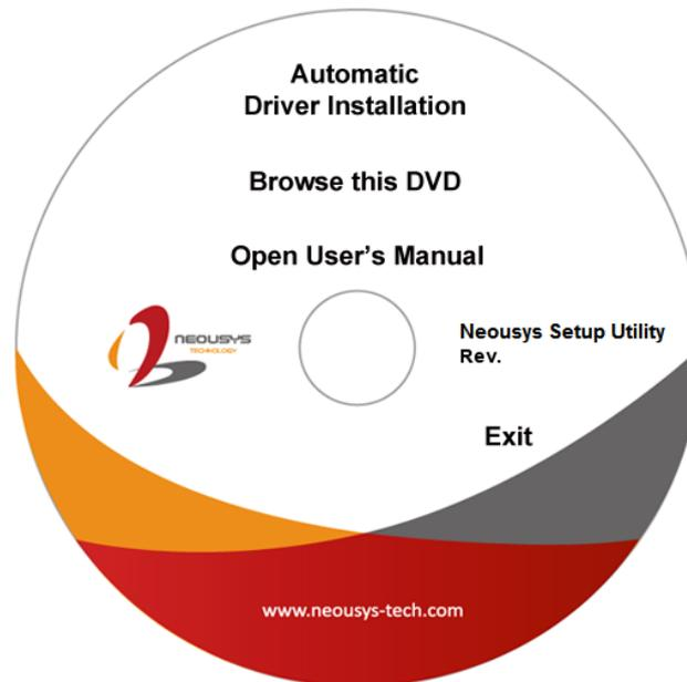
2. Click on “**Automatic Driver Installation**” and the setup utility will automatically detect your Windows operating system and install all necessary drivers. The installation process takes about 6~8 minutes depending on your Windows version. Once driver installation is done, the setup utility reboots your Windows and you may begin using your system.
